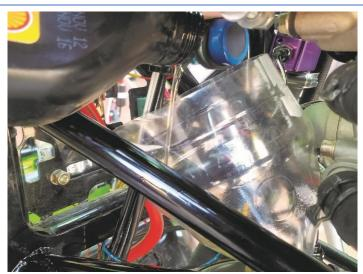
Re-Check the Dipstick that the Oil Level is up to the full mark at the top of the Dipstick.
