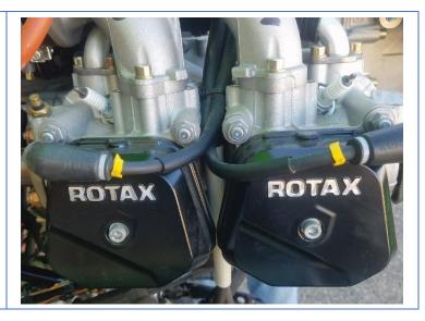
7 Lift up on the Oil Reservoir quick drain to release Oil into your receptacle.
