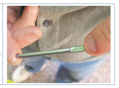
Remove & inspect the Magnetic Plug.
