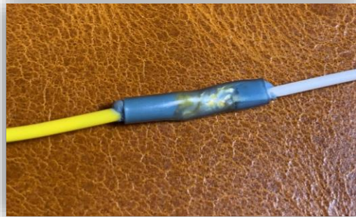
PHOTO 5: Solder Sleeve with Meltable Ring now “melted”. Clearly, the “ring” visible as a shade of red in the prior photos has liquified & become the solder/binder creating connectivity between the 2 wires. The red dye is no longer visible.
